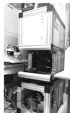
Fig. 10 YAG Laser for Laser Ablation in Liquid (LAL) Sampling
