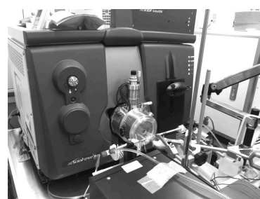
Fig. 7 Organic Mass Spectrometer equipped with in-house Ion Source
